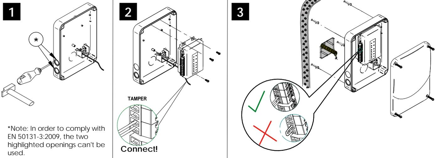
Note: Follow the same connection model, using the CU tamper input, when using a third party electric box equipped with a tamper opening detection.
