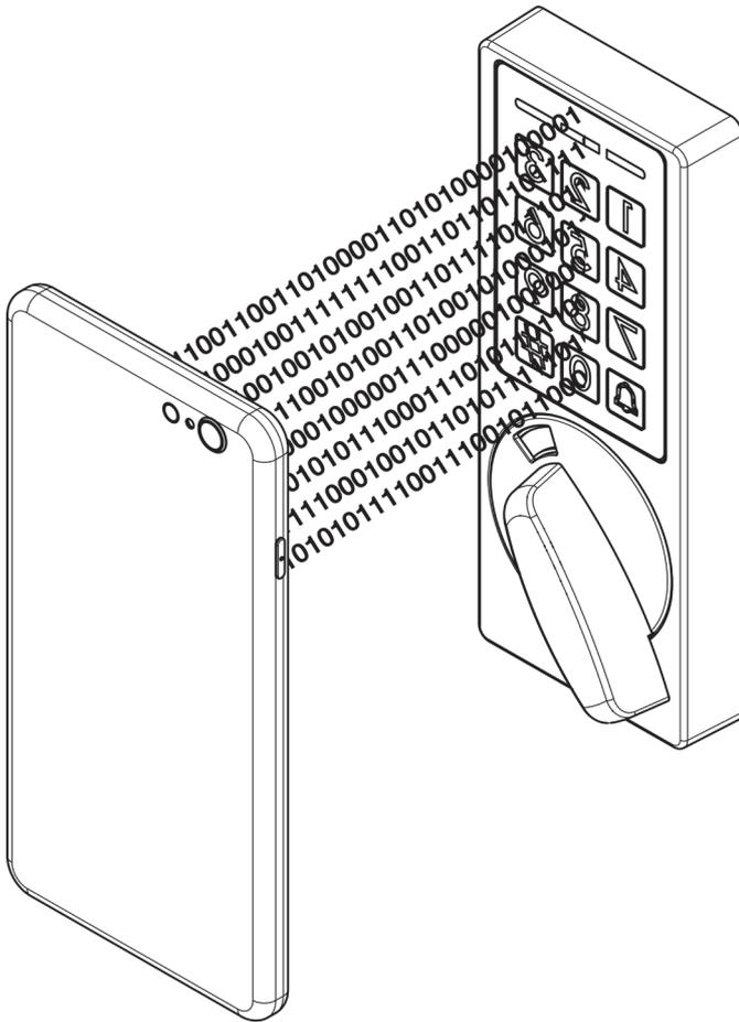
VLC (Visual light communication) is the optical data transmission technology that is used to configure the device for use. It transmits device configuration data and access credentials using your mobile phone or tablet's screen.
