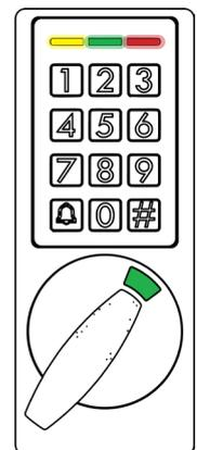
4. Release the button. The keypad will restart. A startup beep sounds and all the LED's blink once. Connect the 'White and Black' pair of cables next to the button if disconnected.
