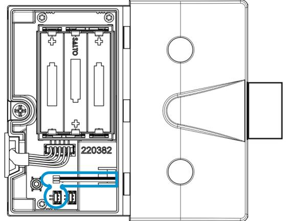
2. Remove one or all the batteries in the battery holder. Push the button above the battery holder and hold it.
